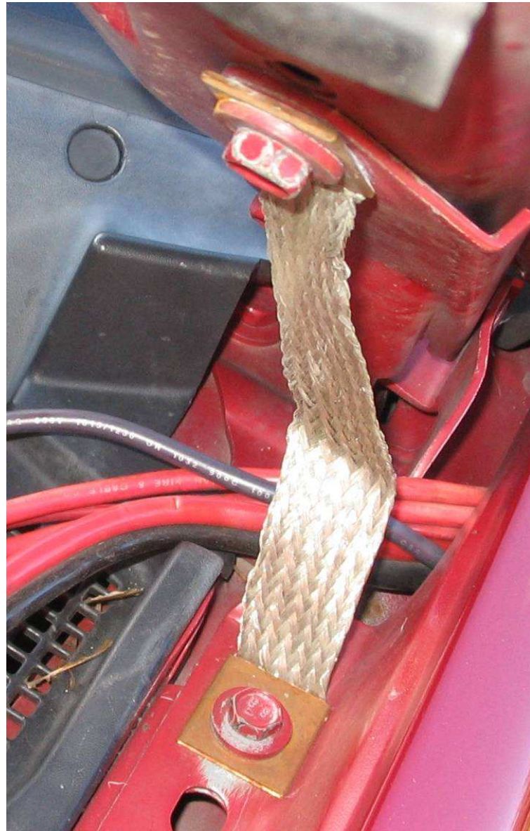
Figure 9: Braid installed to ground the hood to the body on a car.
