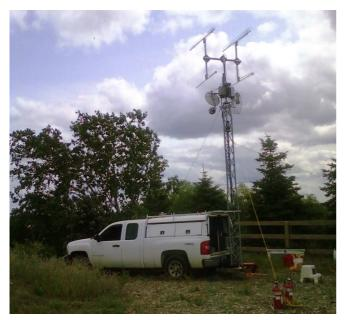
Way up there, are loop yagi antennas for 902, 1296, 2304, and 3456 MHz operation, along with parabolic dish antennae for the 5760 and 10368 MHz bands. In addition to a standard rotator to turn the array of antennae to any compass bearing, there is an elevation rotator up near the top, so that the dishes can be pointed precisely in not only the azimuth direction, but the elevation direction. This is critical for these extremely high
