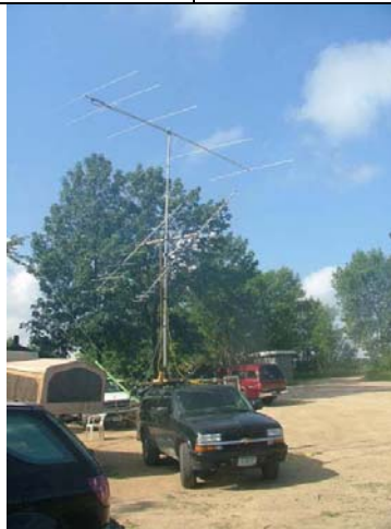
6 Meter VHF beam at the top, and elevatable 2 M and 70 cm beams below that, tipped up for a satellite pass.
