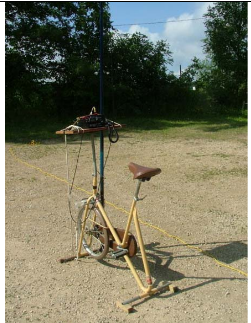
For additional ARRL bonus points, we needed some QSO's made with totally natural power. So we have a generator on the exercise bike connected to a QRP radio. How many watts can you pedal today?
